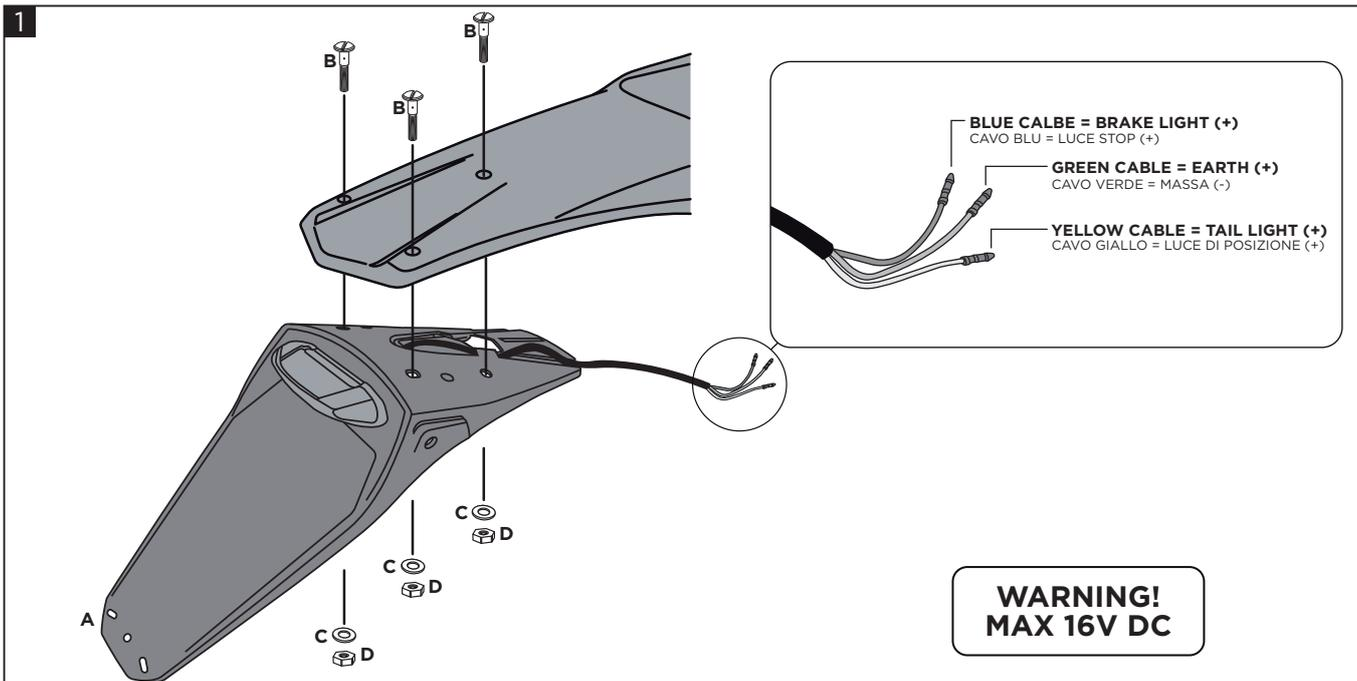
**Place the license plate holder under the rear fender and drill it in the points shown above. Connect the power cables as shown, then tighten the license plate holder to the rear fender using bolts (B), washers (C) and nuts (D).**
