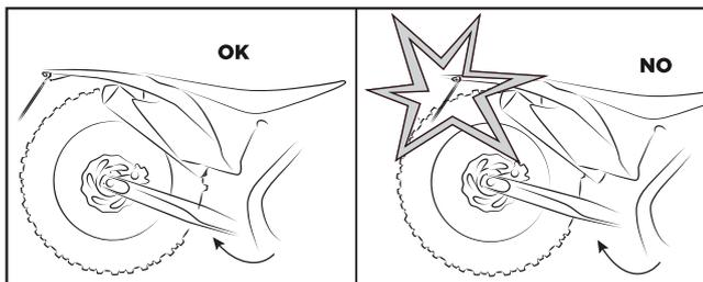
**ATTENTION: check that the license plate holder doesn't touch the wheel when the shock absorber reaches its limit switch.**
